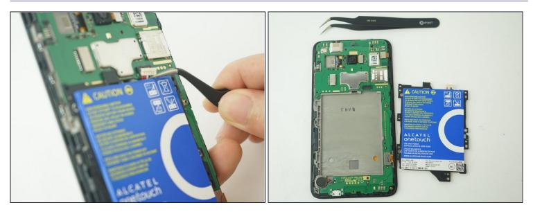
• Use a pair of <u>tweezers</u> to pull the battery connector from its port.
