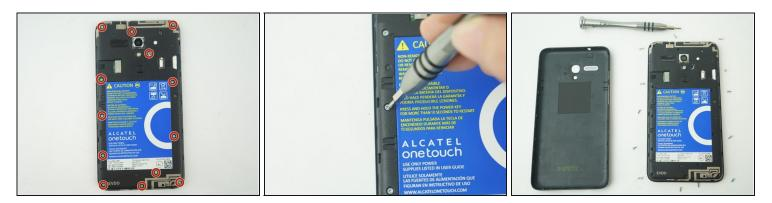
• Remove 13 1mm JIS screws with JIS #000 Screwdriver.
