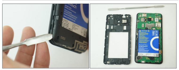
• Gently pry off the Mid frame from the phone using a Metal Spudger.
