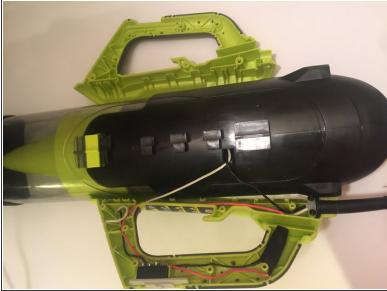
After all 9 screws have been removed, seperate the handle housing the on/off switch.
