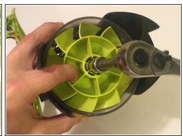
• Remove new fan from package and install as shown. Screw the nut back on to secure the fan. Remember the nut is reverse thread, so turning it counter clockwise will tighten it. The fan will also need to be secured while the nut is being tightened.
