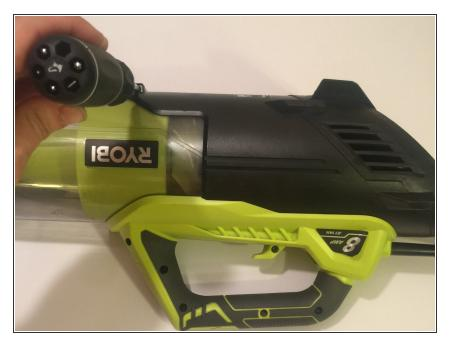
Using a T15 torx drive(star-head), carefully remove each of the 9 screws and set aside in a secure location. All 9 screws are 10 mm long.
