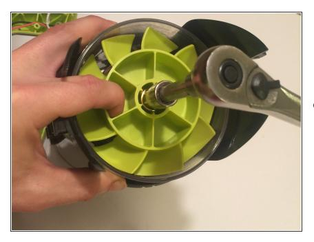
Once the blower shaft is detached, the fan will be visible. Use a ratchet with a 1/2" socket to remove the 1/2" nut securing the fan to the motor. This nut is reverse thread so turning it clockwise will loosen it. The fan will also need to be secured so that it does not spin as the nut is being loosened.
