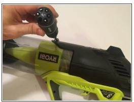
Slide blower shaft back into motor housing, close handle back around blower shaft and motor housing, and screw all 9 screws back into their location.
