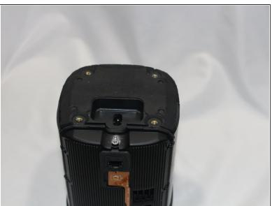
Slide the protective cover upwards to remove.
