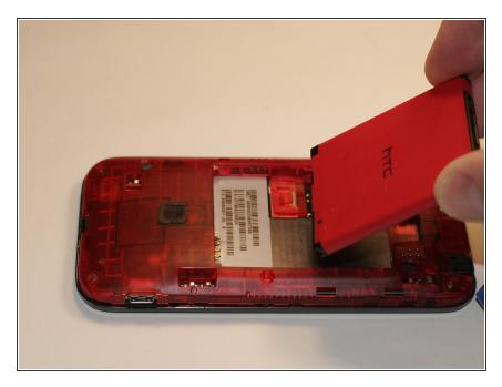
Remove the red battery to replace.
