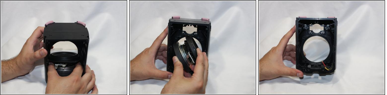
**i** The woofer is snugly fit into the frame socket, some careful manipulation is required to remove the woofer from the housing.
