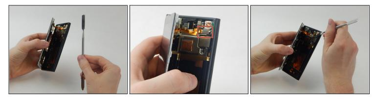
• Wedge a spudger underneath the silver rectangle in the upper right corner until it pops off the back of the phone.
