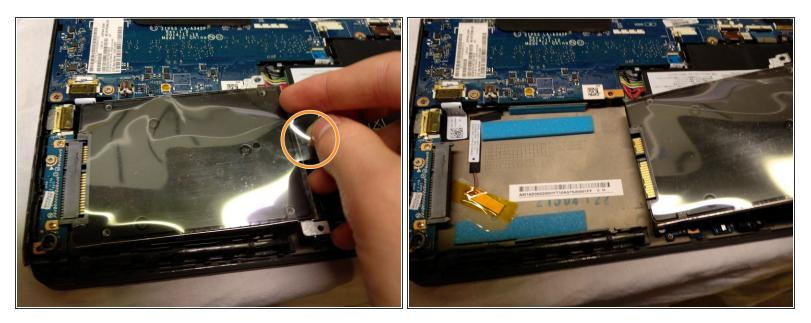
• Gently grab the plastic tab. Lift and pull the SSD assembly out of the computer
