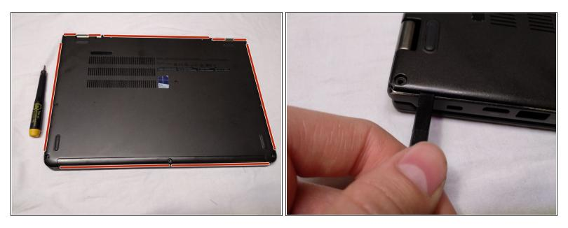
• Pry up the case carefully using a spudger.
