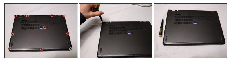
Remove the ten Phillips screws using a Philips 00 screwdriver
