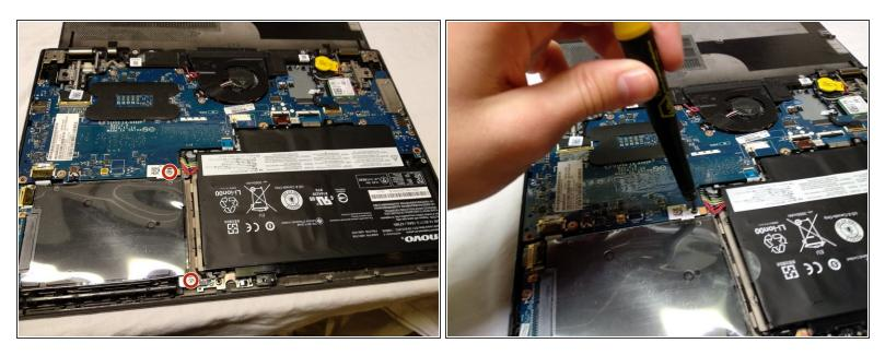
Carefully remove two Phillips screws with a Phillips 0 screwdriver
