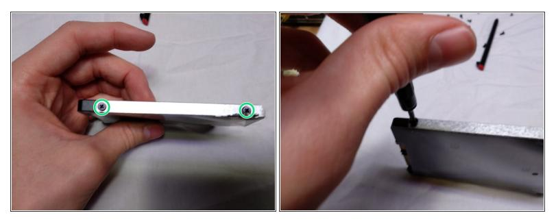
• Remove the 4 identical Phillips screws with a Phillips 00 screw driver (they are on both sides).
