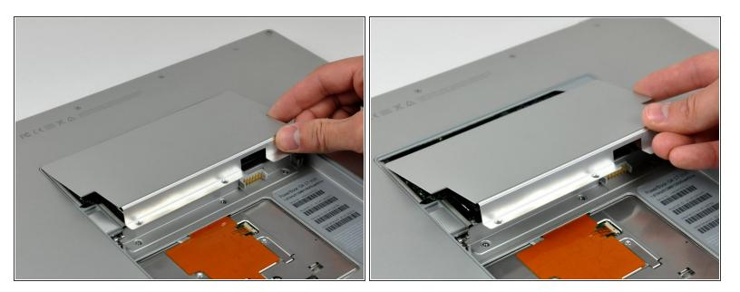
• Lift the memory cover slightly and pull it toward yourself to remove it from the lower case.
