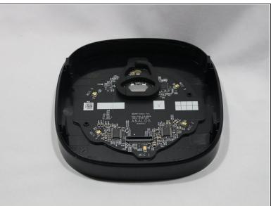
Pull the control panel away from the speaker to separate.
