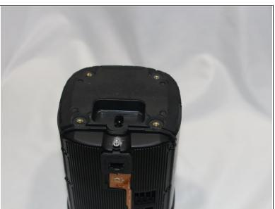
Slide the protective cover upwards to remove.
