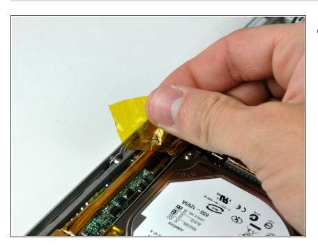
If necessary, remove the strip of tape covering the speaker cables.
