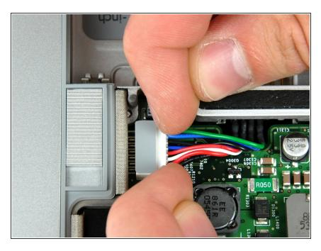
Disconnect the battery cable connector straight away from its socket on the logic board.
