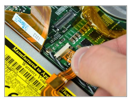
Pull the PRAM battery & USB board cable out of its socket.
