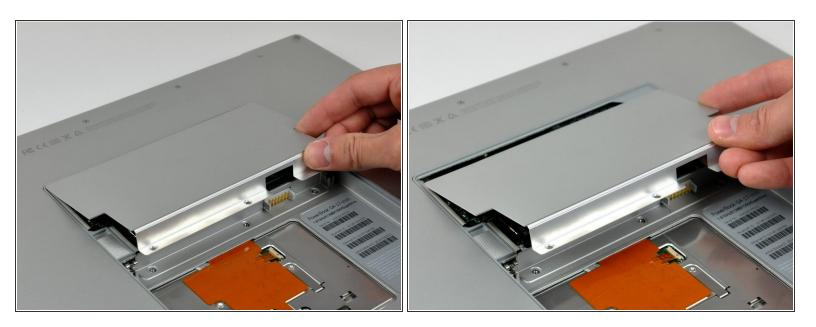
Lift the memory cover slightly and pull it toward yourself to remove it from the lower case.
