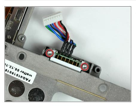
Remove the two 8.5 mm T8 torx screws securing the battery connector to the lower case.
