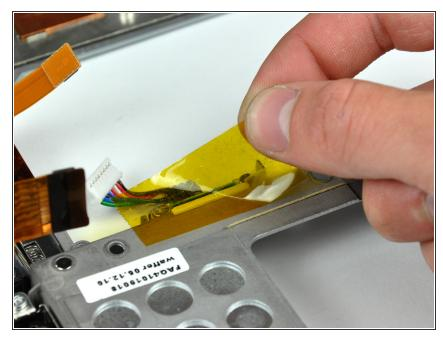
if necessary, peel the yellow Kapton tape covering the battery connector.
