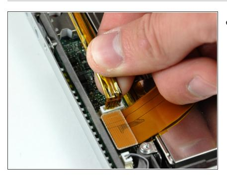
Pull the speaker cable straight up to disconnect it from the sound card.
