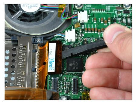
Use the flat end of a spudger to pry the PC card cage cable connector up off the logic board.
