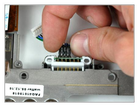
Gently pull the battery connector away from its housing in the lower case.
