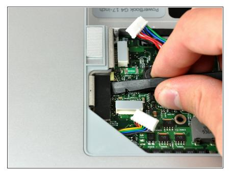
Use the flat end of a spudger to pry the AirPort/Bluetooth cable connector up off the logic board.
