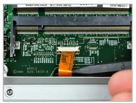
Use the tip of a spudger to slide the trackpad ribbon cable out of its socket.
