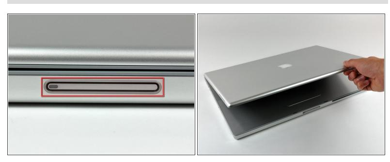
Depress the display latch release button and open your display.
