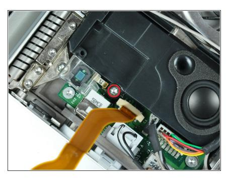
Remove the single 6.9 mm T8 Torx screw securing the left speaker to the lower case.
