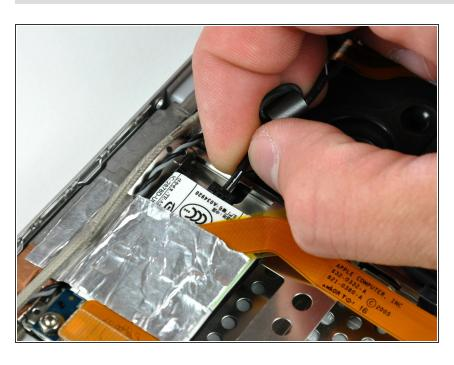
Disconnect the RJ-11 cable from the modem.
