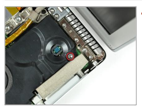
Remove the single T8 6.9 mm Torx screw securing the right speaker to the lower case.
