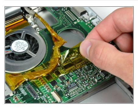
If necessary, remove the piece of tape securing the display data cable to the logic board.
