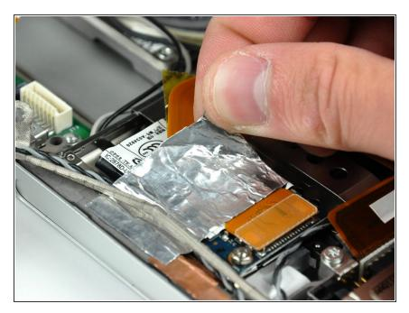
Peel back the piece of foil tape covering the modem cable to free the speaker cable held underneath.
