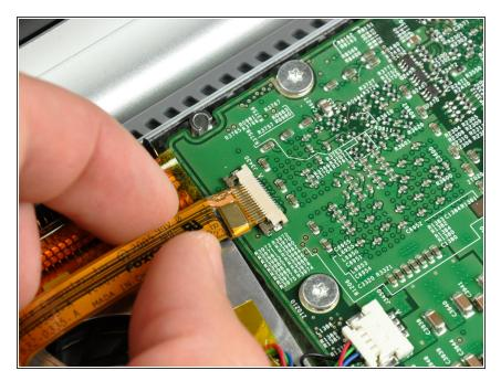
Pull the DC-in ribbon cable straight away from its socket.
