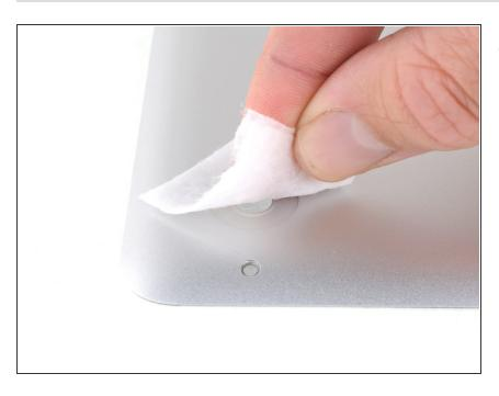
Scrub the foot pad with adhesive remover to remove any remaining adhesive.
