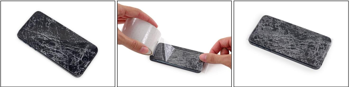
**i** If your display glass is cracked, keep further breakage contained and prevent bodily harm during your repair by taping the glass.
