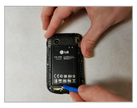
Pry the battery out of the device with a plastic opening tool and remove it.
