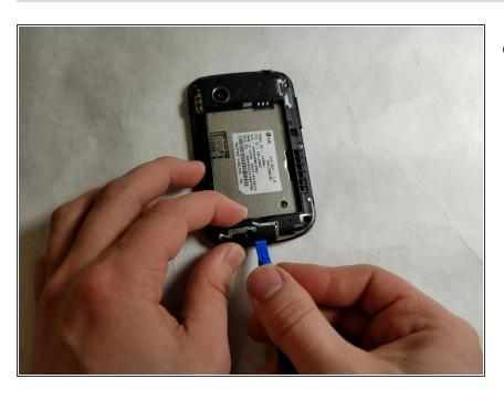
Pry open the bottom part of the internal casing with the plastic opening tool and remove it.
