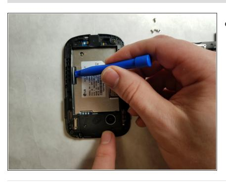
Pry open the top part of the internal casing with the plastic opening tool and remove it.
