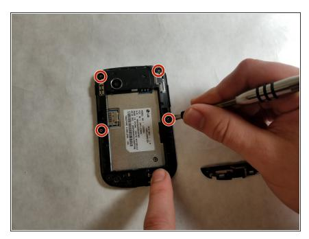
Remove the four 4 mm screws using a JIS screwdriver with a J000 head from the top part of the internal casing.
