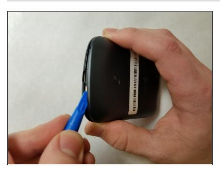
Pry open the back case on the device with a plastic opening tool and remove it.
