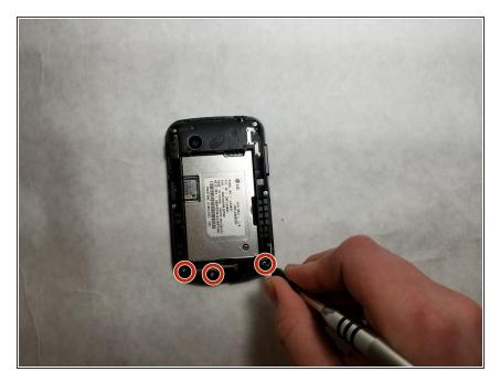
Remove the three 4 mm screws using a JIS screwdriver with a J000 head from the bottom part of the internal casing.
