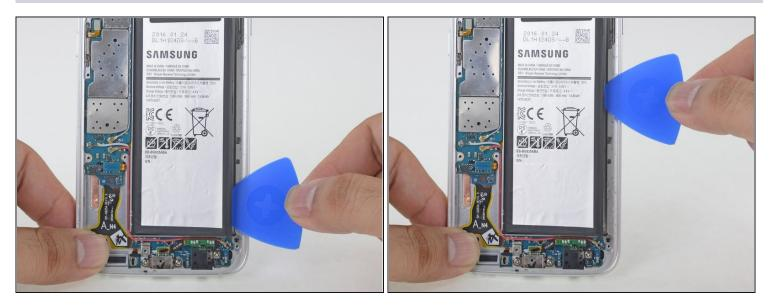
• Slide the opening pick up the side of the battery to break apart any remaining adhesive.
