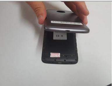
• Insert the spudger into the notch on the corner of the phone and lift up to remove the back case.
