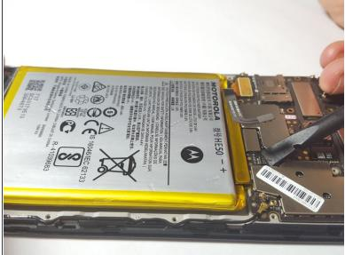
After removing the back panel, use the spudger to lift and detach the <u>Battery Flux Cable</u> from the <u>Motherboard</u>.
