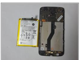
Wedge the spudger between the battery and the phone to lift the battery up and remove the battery. There will be slight resistance to this but the battery will not be damaged by this. It is just the adhesive tape.
