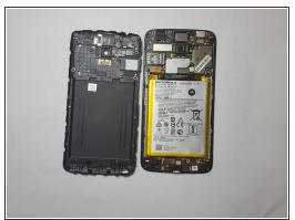
Lift up and remove the back panel.
