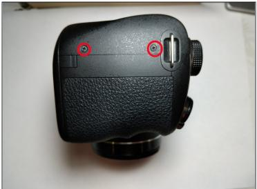
Remove the four 6mm Phillips #00 screws.
