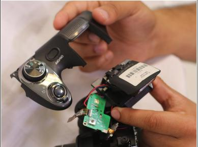
Slide the flash out and away from the camera to remove.
