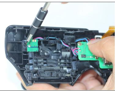
Remove the four 6mm Phillips #000 screws from the bottom of the case.
