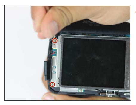
Remove the two 6mm Phillips #000 screws.
