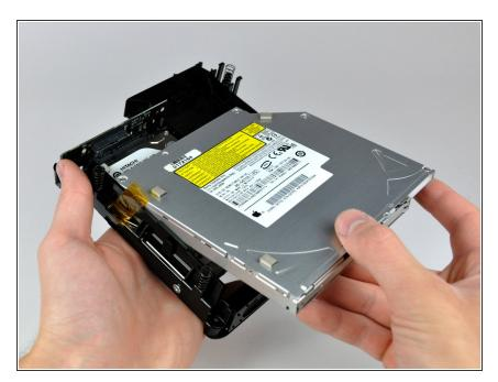
Gently lift the optical drive out of the internal frame.
