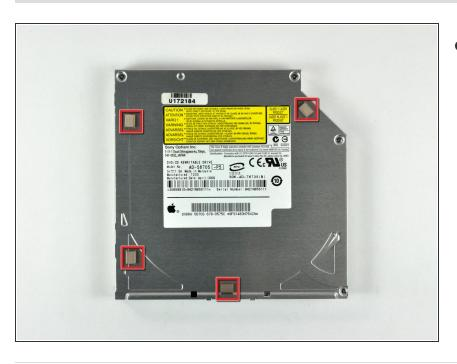
Transfer the four foam bumpers to the replacement optical drive.
