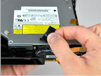
Use the tip of a spudger to remove the black electrical tape spanning the interconnect board and optical drive.
