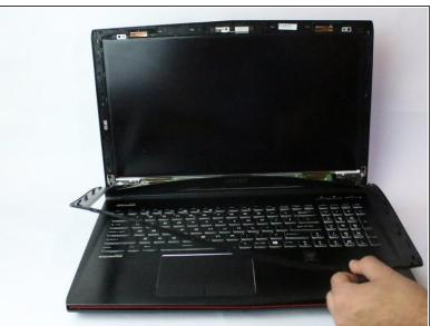
• Once it has started to separate, gently pull off the screen panel by working along the edge, and set it aside.
