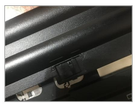
Push the switch into the unlock position. Pull the battery out.
