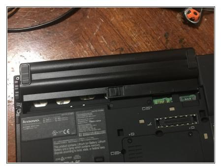
Position the new battery in the same manner as the old battery (with the connectors and lock/unlock switch facing inwards towards the computer). Push the battery in.
