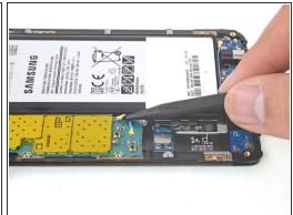
Use the point of a spudger to disconnect the two antenna cables.
