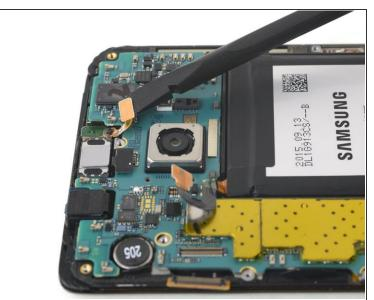
Use the flat end of a spudger to disconnect the front-facing camera ribbon cable.
