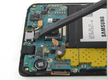
Use the flat end of a spudger to disconnect the front-facing sensor array ribbon cable by prying it straight up from its socket.
