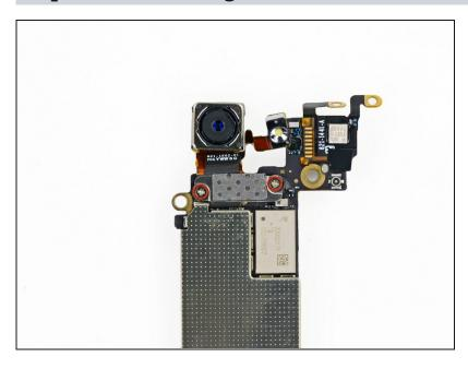
Remove two 1.1 mm Phillips screws securing the rear-facing camera bracket to the logic board.
