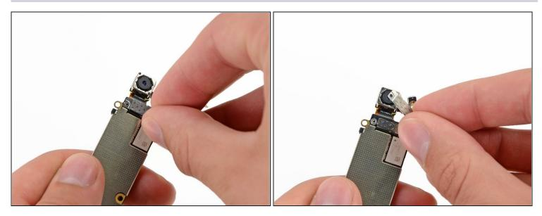
• Remove the rear-facing camera bracket from the logic board.
