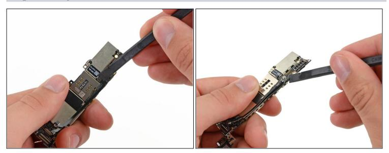
• Use the flat end of a spudger to disconnect the bottoms of the interconnect cables from their sockets on the logic board.
