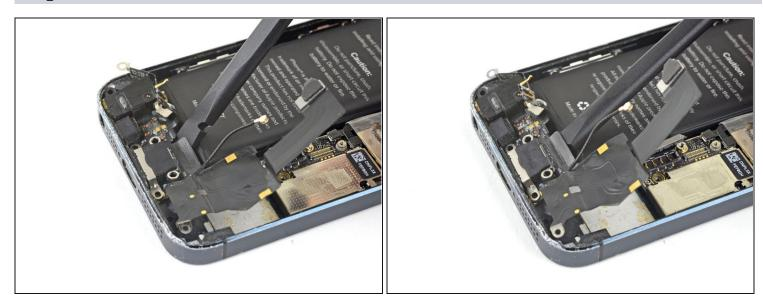
• Use the flat end of a spudger to loosen the rest of the Lightning connector assembly from the rear case.
