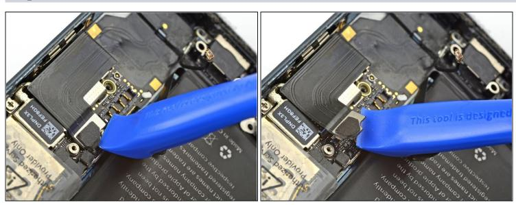
• Use the opening tool to pry up and disconnect the Lightning connector cable connector from its socket on the logic board.
