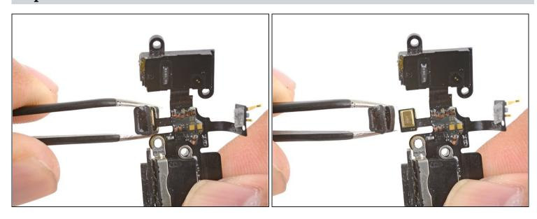
• Use <u>tweezers</u> to gently pull and remove the rubber microphone sleeve off of the microphone. Transfer the sleeve onto the replacement part.
