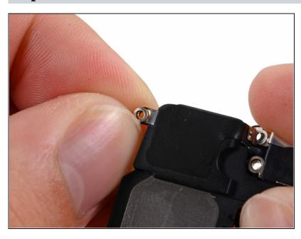
Remove the small double-sided metal washer on the speaker enclosure and transfer it to the replacement part.
