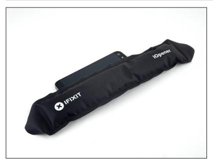
Flip the phone face up, heat an iOpener, and apply it to the right edge of the phone for a minute.
