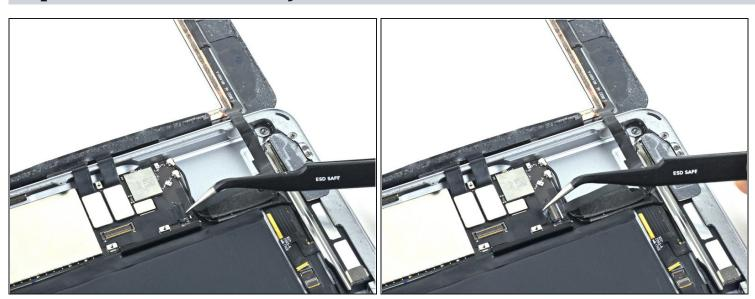
• Remove any tape covering the home button ribbon cable connector.
