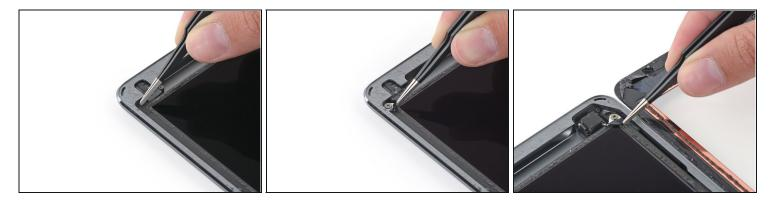
• Remove any tape obscuring the LCD screws.
