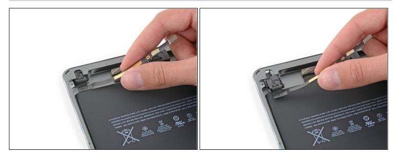
• Use the headphone jack cable to gently remove the headphone jack from its recess in the case.
