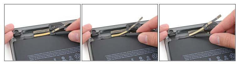
• Slide the flat end of a spudger under the headphone jack cable to free it from the adhesive securing it to the rear case.
