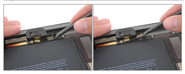
• Use the flat end of a spudger to lift the headphone jack cable connector straight up from its socket on the logic board.
