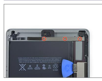
Remove the three 1.4 mm Phillips #000 screws securing the upper component cable bracket.
