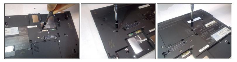
Using a Phillips #00 screwdriver unscrew the four screws in the back of the laptop that have a keyboard symbol next to them.
