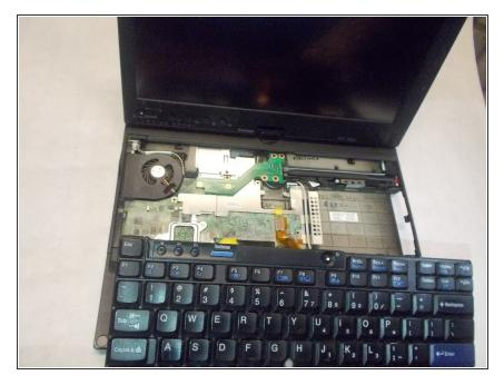
• Use a flathead screwdriver to gently lift up on the keyboard until it comes off. Make sure you disconnect the ribbon cable from the motherboard before removing the KB completely.
