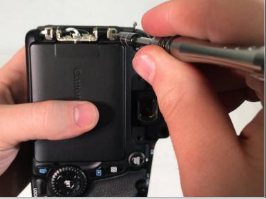
Remove two 4 mm Phillips #000 head screws that mount the LCD touchscreen to the hinge on the camera.
