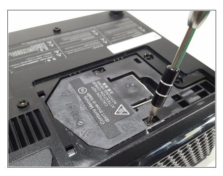
Remove the two screws on the bulb housing.
