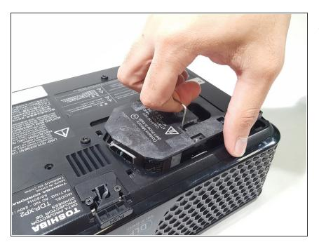
Pull the tab up and pull the bulb out vertically. Some force will be required, but it will come out.
