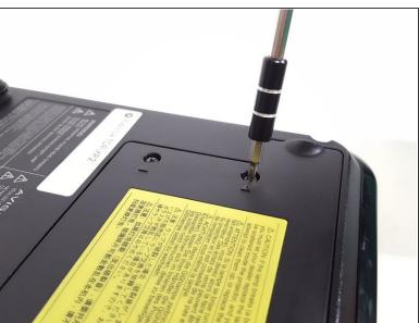
Remove the two screws from the bottom plate as shown.
