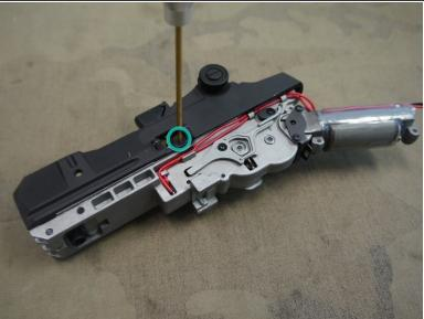
Begin adding the short 2mm screws with the cone shaped heads into the areas shown.
