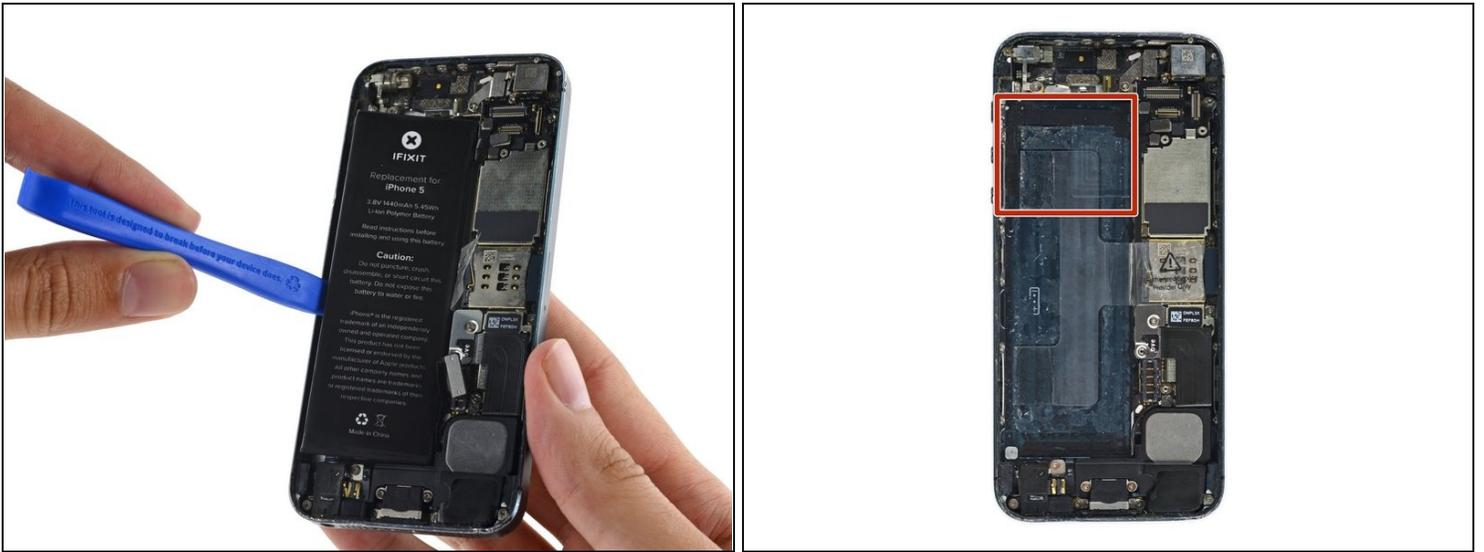
⚠ Use the plastic opening tool to **gently** pry the battery up, **only at the outside edge of the phone**. Prying anywhere else, especially near the logic board, **may result in damage to the logic board**.
