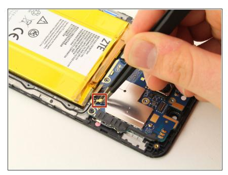
Use tweezers to remove the antenna. The antenna comes up on the right side of the phone, by the battery, and is attached to the motherboard.
