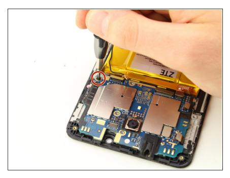
Using the #00 Phillips screwdriver, remove the 3.0 mm screw located on the right edge of the phone, above the battery.
