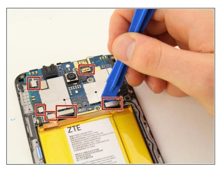
Use the plastic opening tool to remove the connectors on the motherboard.
