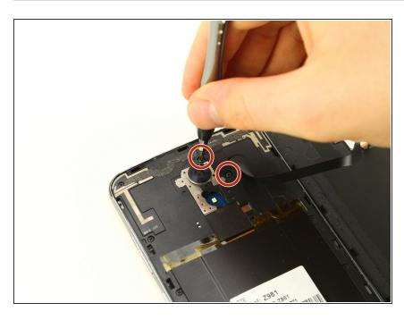
Using the Phillips #00 screwdriver, remove the two 3.0 mm screws located near the top of the phone, next to the rear camera.
