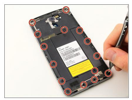
Using the Phillips #00 screwdriver, remove the 15, 3.0 mm rear panel screws located around the perimeter of the phone.
