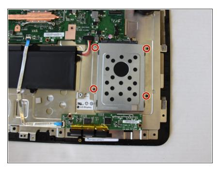
Remove the four 5.0 mm Phillips #1 screws on the outer casing of the hard drive.
