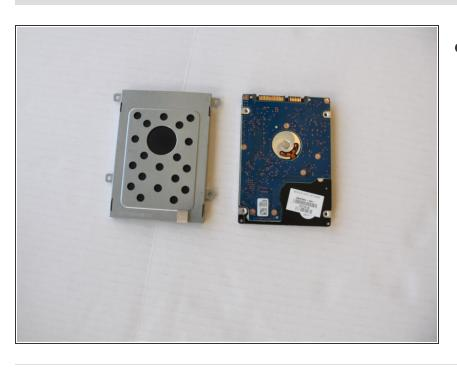
Separate the hard drive from the casing.
