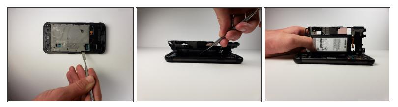
• Use a metal spudger to pull the mid frame and battery off of the motherboard.
