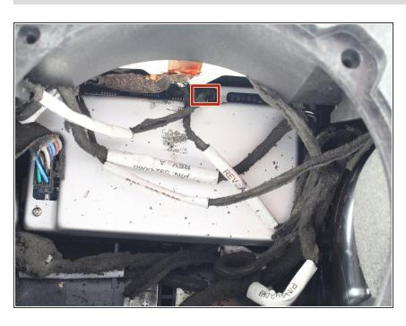
Remove the sensor connection by pulling it straight out with your hand.
