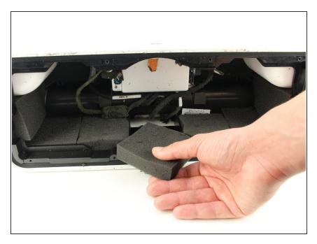
Remove the middle foam panel from the wall of the device closest to you by pulling the foam out with your hand.
