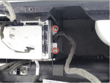
Remove four 2mm Phillips #1 screws from the base of the power supply box by placing the screwdriver in the head of the screw and rotating counterclockwise.
