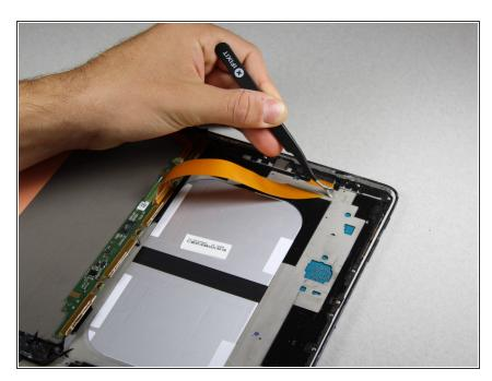
Using the tweezers, gently peel up on the silver tape covering the connector.
