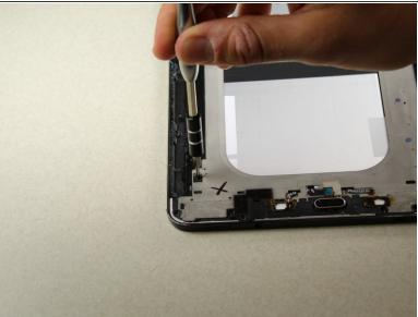
Remove the 2 centrally-located black 3.0 mm Phillips head screws using the screwdriver.
