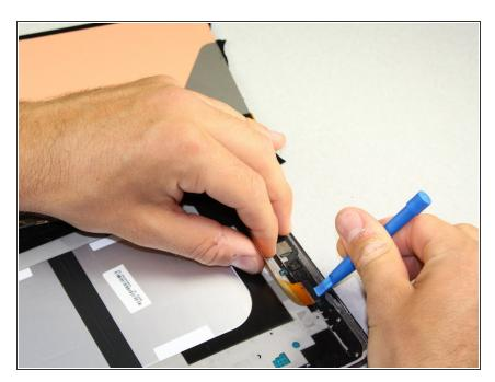
Use the plastic opening tool to get under the connector piece. This will allow you to remove the front panel assembly from the rest of the device.
