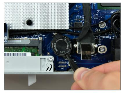
Use the tip of a spudger to pry the PRAM battery out of its socket.
