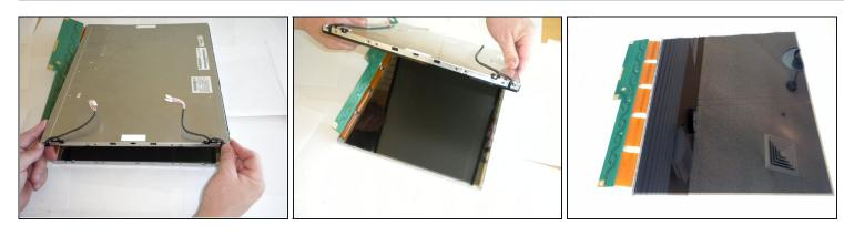
• Lift the LCD back cover to reveal the LCD screen below.
