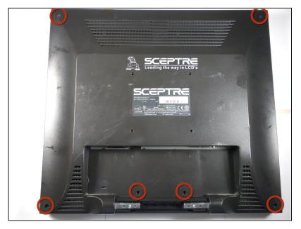
Using a #2 Phillips screwdriver, remove the six 7mm screws at the circled locations.
