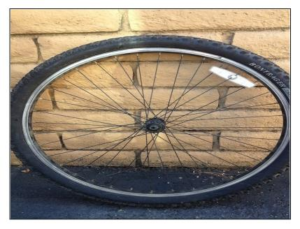
• After the quick release lever is removed, the wheel can be separated from the front fork.
