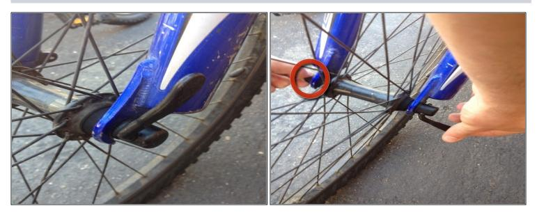
• Find the quick release lever on the outside of the bike's fork on the right hand side. Flip the lever down and turn the lever counter clockwise, loosening the lever until it comes off.
