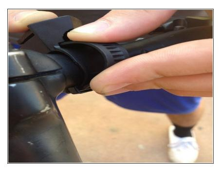
Pull the strap tightly through the clasps at the bottom of the mount.
