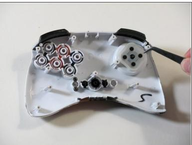
Insert a new directional pad over the original directional pad's location.
