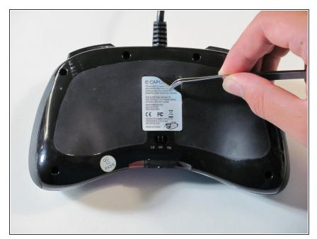
Use tweezers to completely remove the sticker from the rear of controller.
