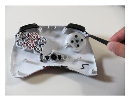
Use tweezers to remove the rubber part of the directional pad.
