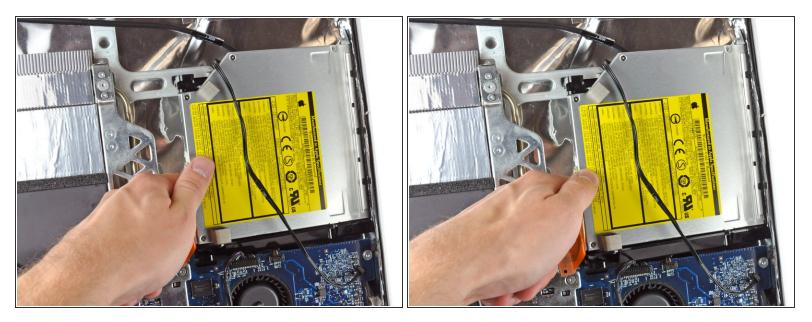
• Reach behind the chassis and use your finger to unclip the lower optical drive tab from the chassis.
