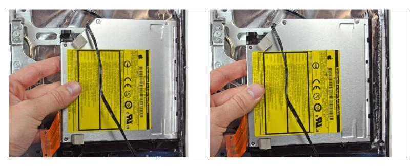
Maneuver the optical drive out of the rear case, minding the two plastic pins molded into the rear case near the open end of the optical drive that can break off.
