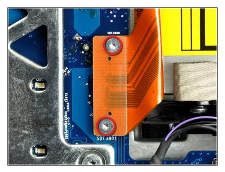
Remove the two 3.6mm T6 Torx screws securing the optical drive ribbon cable connector to the logic board.
