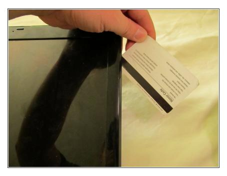
Slide a credit card along the edges of the bezel to lift the bezel away from the LCD.
