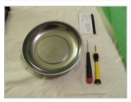
Here is your arsenal of tools. Credit Card, Small flat heat screwdriver, small phillips screwdriver, and a magnet bowl for keep track of screws (you can use the stick side of duct tape or sticky notes).
