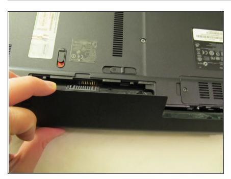
Remove the battery by sliding the clips to "unlocked."
