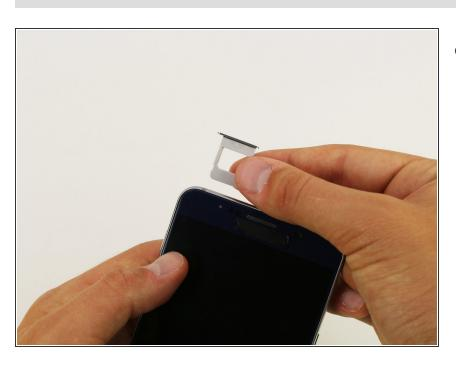
Remove the SIM Card Tray from the slot.
