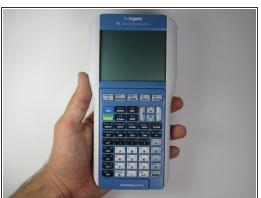
Slide the keypad directly into where it connects to the calculator until you hear a click. Readjust as necessary.
