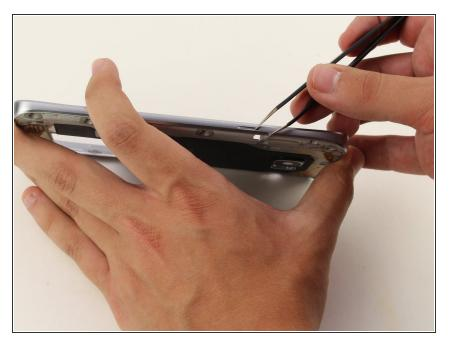
• Push out the power button with the tip of the tweezers.
