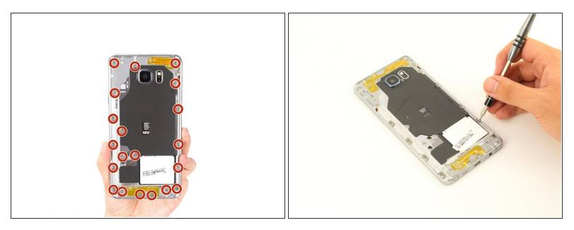
• Remove 20 5mm screws with a Phillips #1 Screwdriver.
