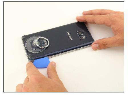
Keeping the pick under the rear glass, move the pick along the bottom edge of the device to cut the adhesive.
