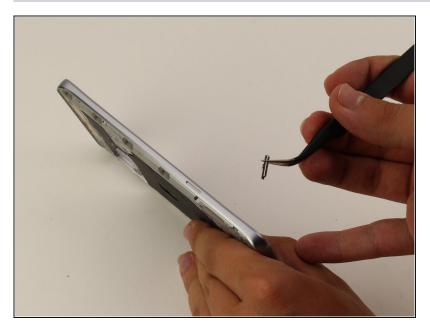
Push out the volume button and remove it from the device.
