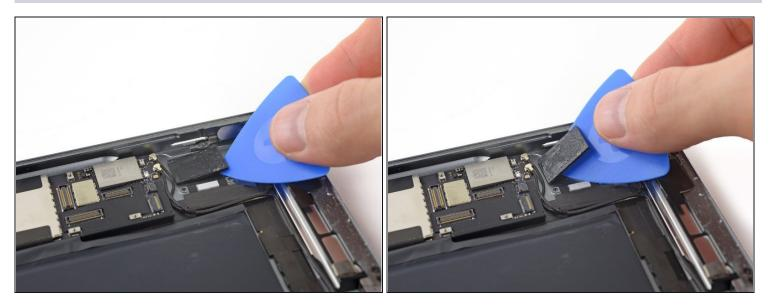
i The SIM board is held to the rear case with a thick adhesive pad.
