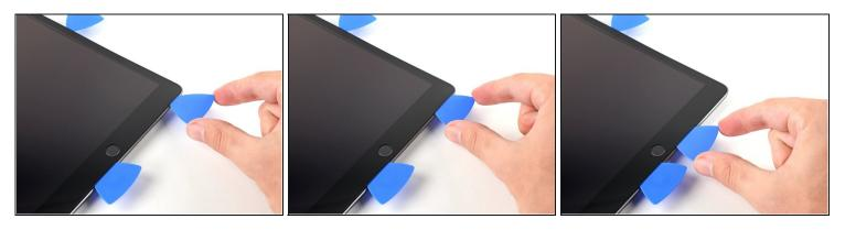
• Re-insert the pick and slide it towards the home button to completely separate the bottom adhesive.
