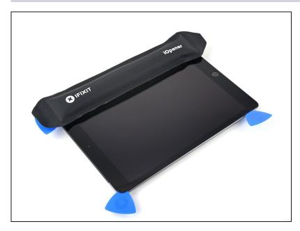
• Heat an iOpener and apply it to the right edge of the device for two minutes.
