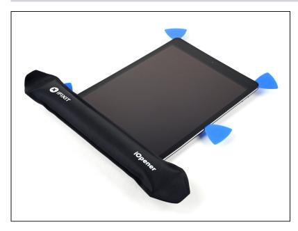
• Heat an iOpener and apply it to the bottom edge of the device for two minutes.
