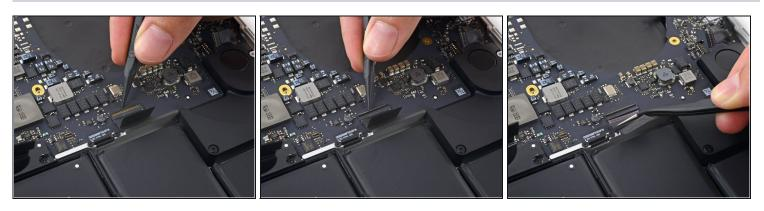
• Use the tip of a spudger to flip up the retaining flap on the keyboard data cable ZIF socket.
