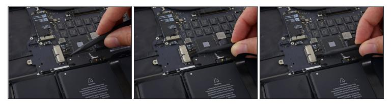
• Use the tip of a spudger to pry the right speaker connector up and out of its socket on the logic board.
