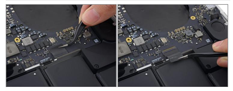
• Peel back the tape covering the top of the keyboard data cable connector.
