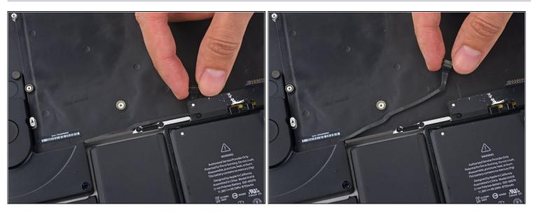
(i) The right speaker cable is lightly adhered to the upper case.
