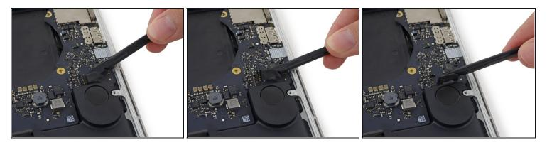
• Use the flat end of a spudger to pry the left speaker connector up and out of its socket on the logic board.
