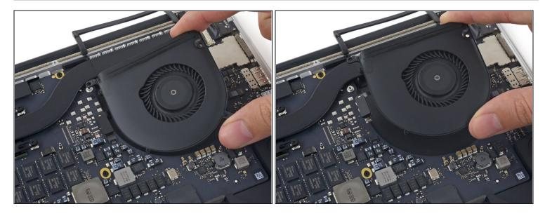
• Lift the fan and push it gently towards the back edge of the MacBook to free the fan cable from its socket.
