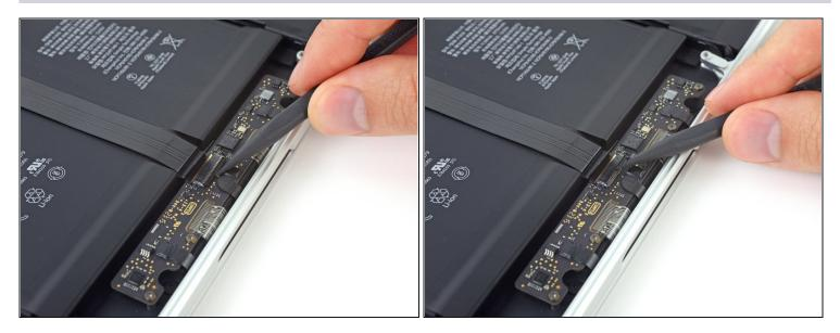
• Use the tip of a spudger to flip up the black locking tab on the trackpad ribbon cable ZIF connector.
