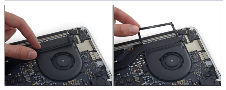
• Peel the left rubber cover up off the fan and fold it out of the way.
