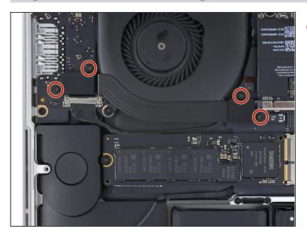
Remove the four 2.2 mm T5 Torx screws securing the I/O board cable connector covers.
