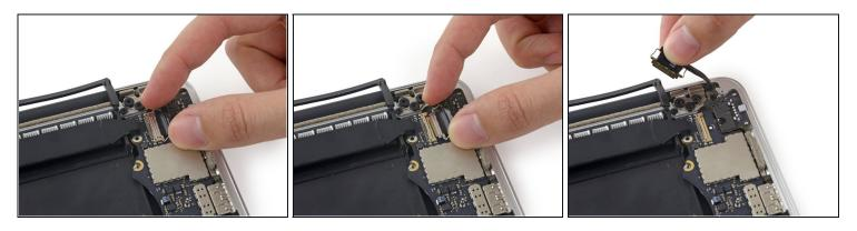
Pull the display data cable straight out of its socket on the logic board.
