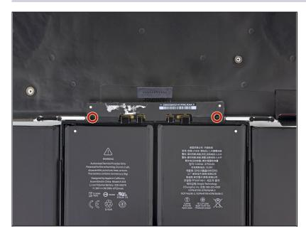
• Remove the two 3.2 mm T5 Torx screws securing the battery board.
