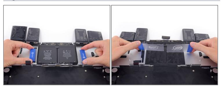
• With one plastic card underneath each of the two center battery cells, twist and lift both cards to fully separate the battery cells, together with the plastic frame and battery board, from the MacBook Pro.
