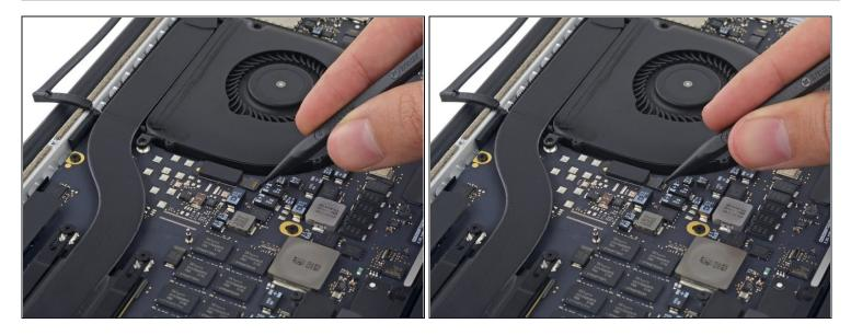
• Use the tip of a spudger to flip up the retaining flap on the left fan ribbon cable ZIF socket.
