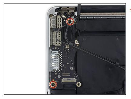
• Remove the two 3.1 mm T5 Torx screws from the I/O board.
