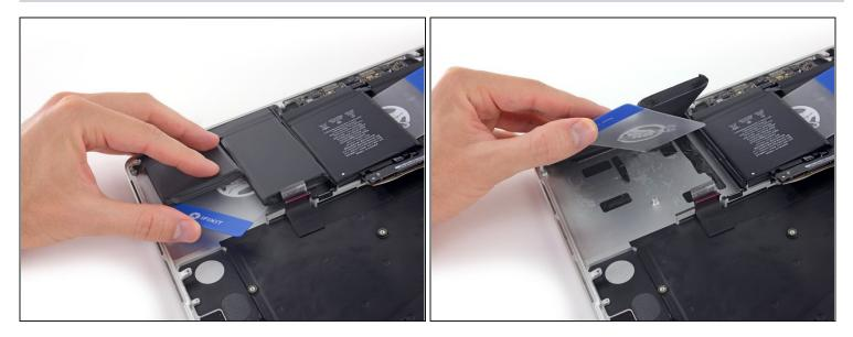
• Flip the two de-adhered right-hand battery cells over the front edge of the MacBook Pro, if you haven't already. This will allow access to the outside edge of the center cell.
