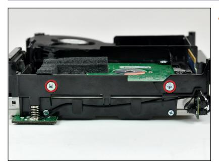
Remove the two Phillips screws securing the side of the hard drive to the internal frame.
