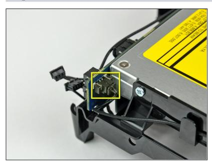
• Use a pair of <u>tweezers</u> or your fingernails to disconnect the speaker cable connector from the interconnect board.
