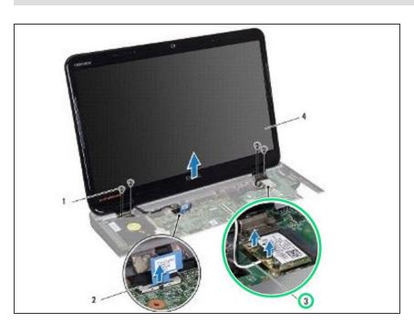
Disconnect the Mini-Card antenna cables from the Mini-Card.
